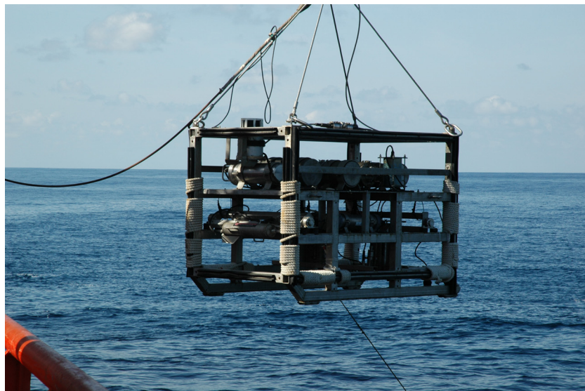
Fig. 8.1: OFOS video sled on deck RV Sonne.
