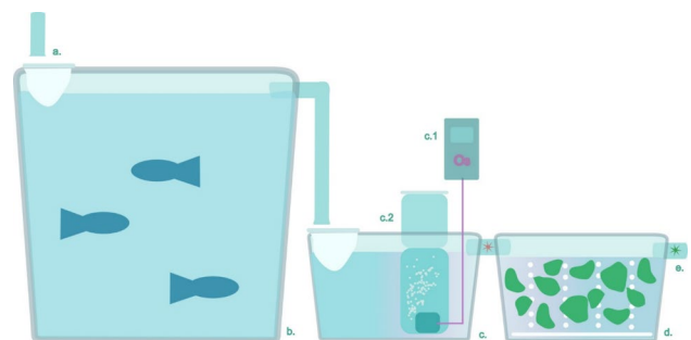
Fig. 1 Experimental setup. The experimental IMTA setup consisted of a. an inlet supplying the system with water pumped from the Ria de Alvor (PT), b. a 450-L conical PVC tank stocked with 18 gilthead seabream ( S. aurata ), c. an 80-L rectangular water treatment unit with c.1. an ozone generator supplied with pure \text{O}_2 and c.2. a protein skimmer mixing the ozone into the effluent water, d. an 80-L seaweed cultivation unit with a perforated plastic tube at the bottom bubbling air for water movement growing U. ohnoi , e. an outlet. The system was operated as a flow-through. Water samples for OPO measurements were taken upstream (red star) and downstream (green star) of the Ulva unit
