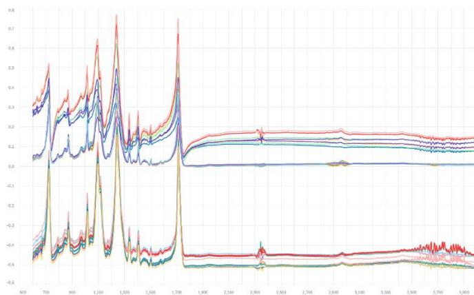
Figure 2 -Spectral changes for Polyethylene terephthalate (PET), in Villefranche, in each season at 7, 60 and 90 days. Figure retrieved from Lenz et al., 2023b.
