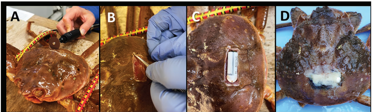
Figure 2. Mounting heart rate logger on snow crab. Carapace abraded above the heart of sedated crab (A), carapace removed from the underlying dermis (B), logger placed in the abraded area of the carapace with electrodes in contact with the tissue (C), logger secured with wax and sealed with quick glue (D).
