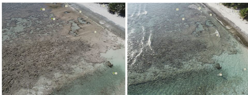
Fig. 7 Visual coastline extraction. An example of aerial images, being used to manually estimate the coastline (yellow lines) in Fig. 3. The images shown here are screenshots from METASHAPE
