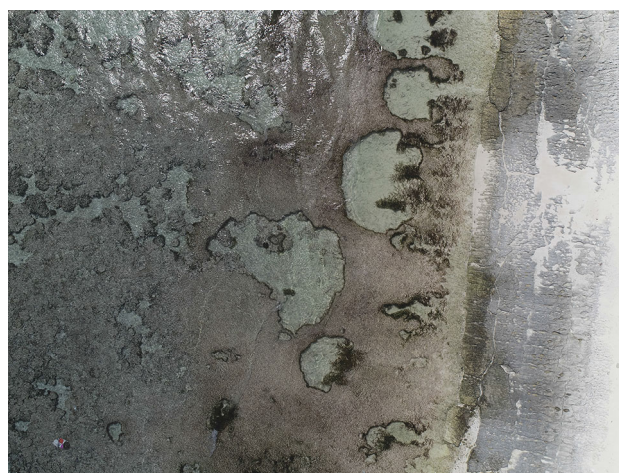
Fig. 6 Sun glint in an aerial image. Sun glint in one aerial image, recorded within flight 4. This type of sun glint also appears on almost all other aerial images of flight 4, showing the water surface. The sun glint is on the images' northwest facing border and thus affects image overlapping within the photogrammetric
